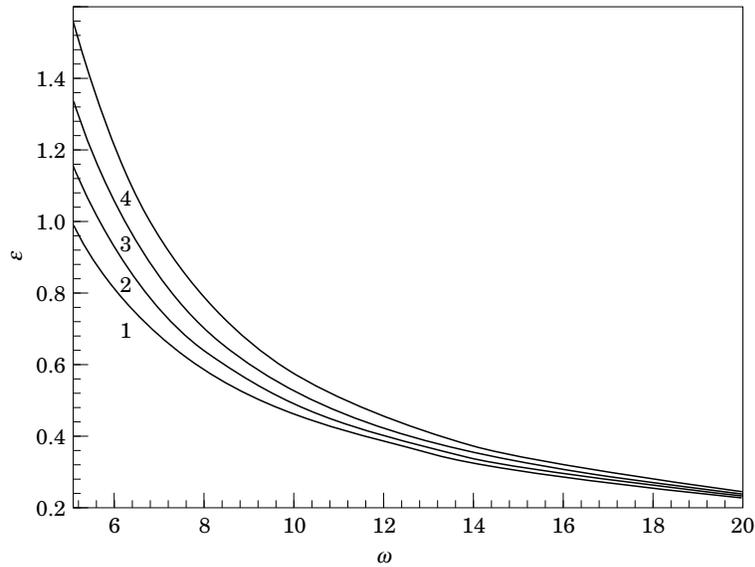
Figure 6. Stability contours: 1,  $c = 0$ ; 2,  $c = 4$ ; 3,  $c = 6$ ; 4,  $c = 8$ .
