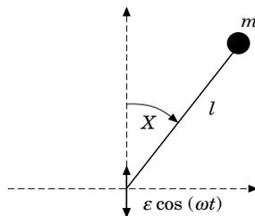
Figure 1. A vertically excited inverted pendulum.
