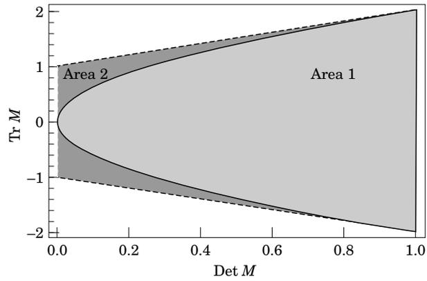
Figure 4. Stable areas for the damped case.
