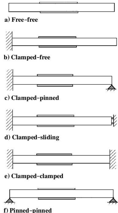
Fig. 2 Beam configurations.
