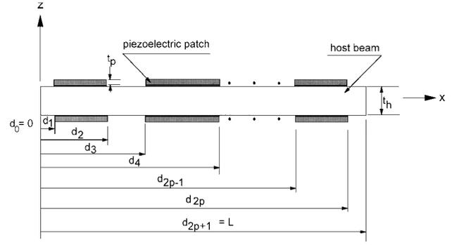
Fig. 1 Geometry of a beam with surface-bonded piezoelectric patches.
