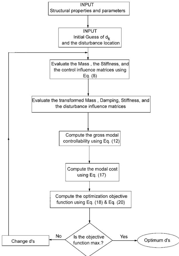
**Fig. 3 Flowchart of the optimization process.**
