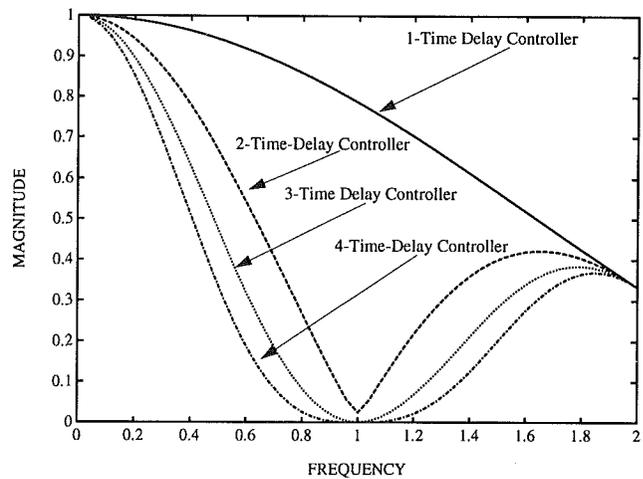
Fig. 7 Magnitude plots of bode diagrams for the time-delay controllers with exact estimated frequency
