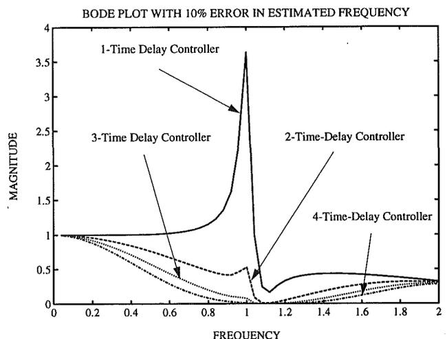
Fig. 8 Magnitude plots of bode diagrams for the time-delay controllers with 10 percent error in estimated frequency
