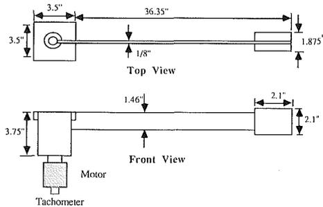
Fig. 2 The flexible link
