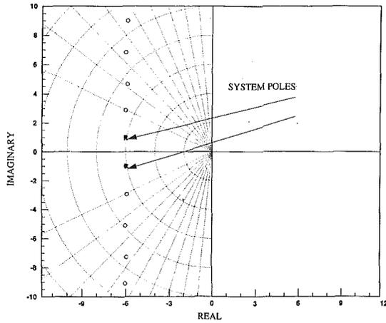
Fig. 2 Pole-zero locations of the controlled system in the  $s$ -plane
