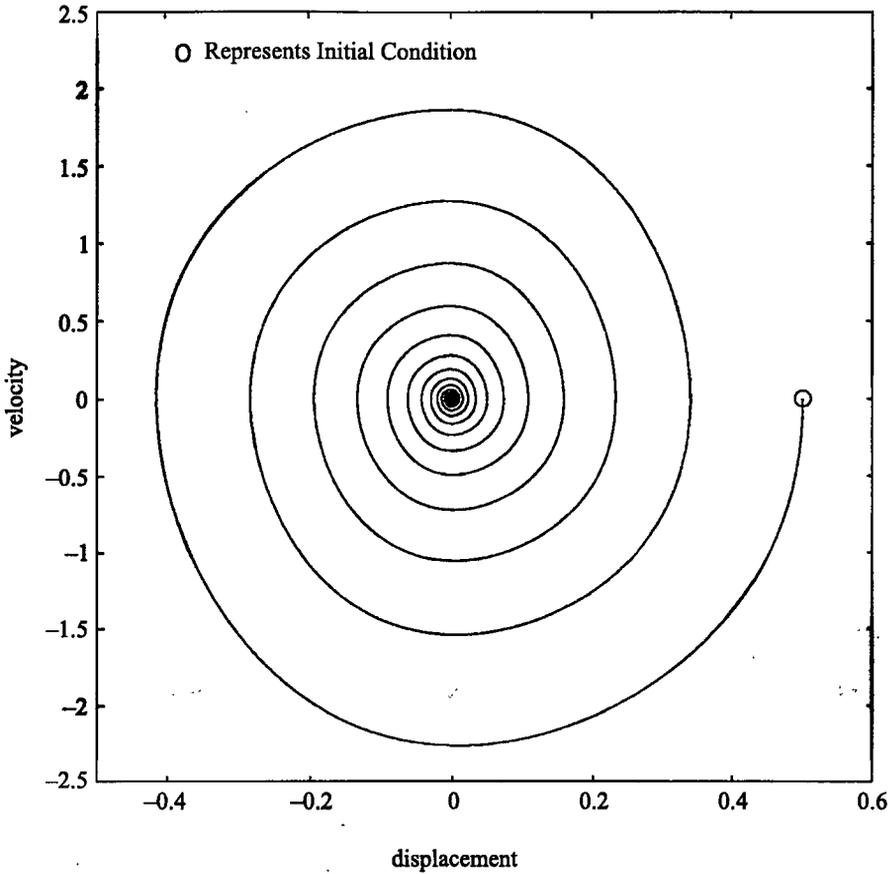
Figure 3. State space of a linear system with a parametric controller.
