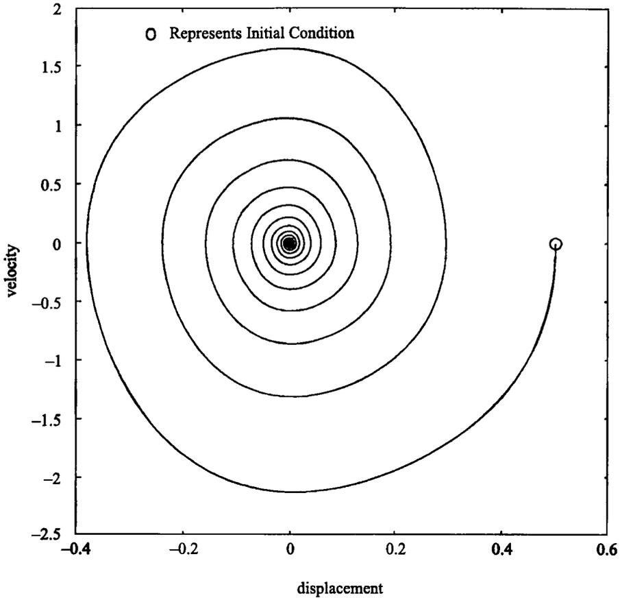
Figure 4. State space of a Vander Pol system with a parametric controller.
