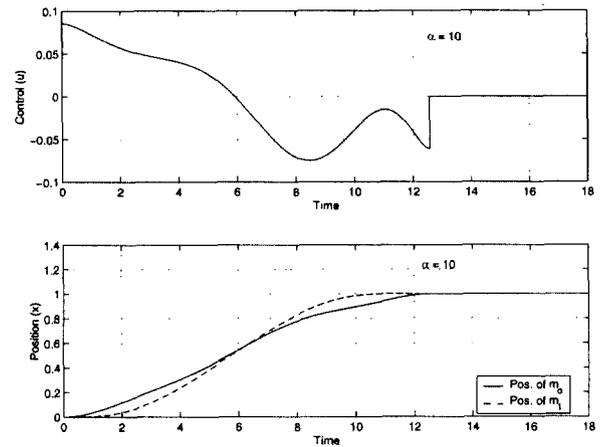
Figure 2: Minimum power/jerk rest-to-rest maneuver.
