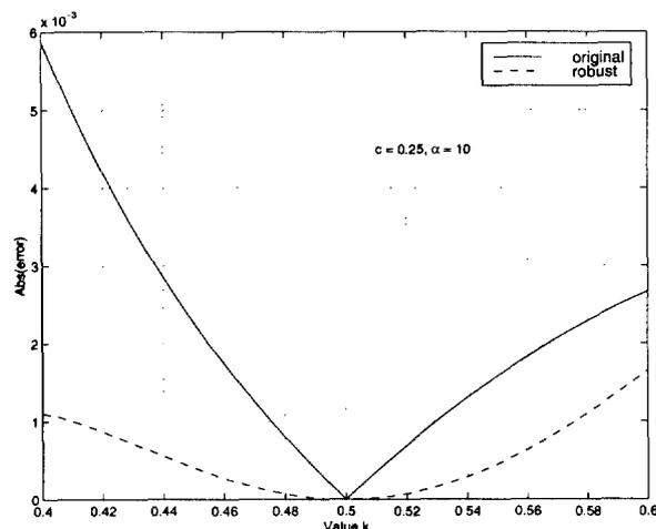
**Figure 4:** Abs(error) at final time vs.  $k$  value for non-robust and robust control
