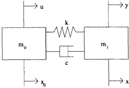
Figure 1: Two-mass/spring/damper system.
