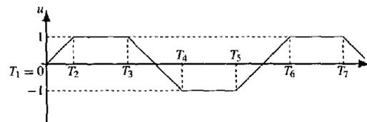
Figure 2. CONTROL PROFILE CORRESPONDING TO JERK PROFILE SHOWN IN FIG. 1
