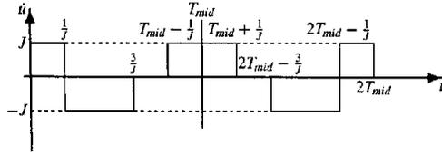
Figure 8. PARTIALLY COLLAPSED JERK PROFILE (CF. 2)
