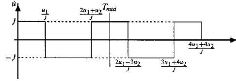
Figure 10. TOTALLY COLLAPSED JERK PROFILE
