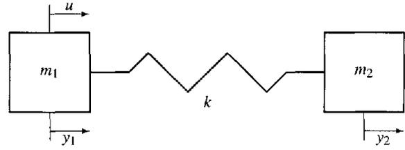
Figure 13. FLOATING OSCILLATOR
