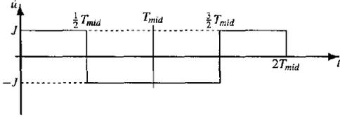
Figure 11. TIME DERIVATIVE OF THE TRIANGULAR CONTROL PROFILE
