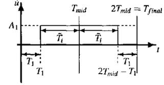
Figure 4. RELATION BETWEEN SWITCHING TIMES FOR AN AXIS-SYMMETRIC CONTROL PROFILE
