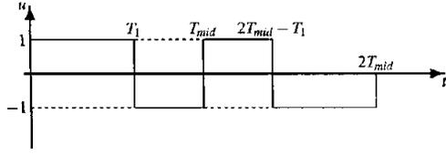
Figure 5. INFINITE JERK CONTROL PROFILE
