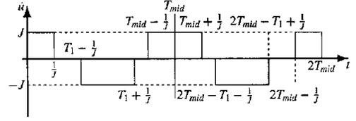
Figure 6. UNCOLLAPSED JERK PROFILE
