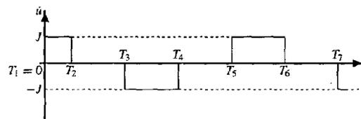
Figure 1. PARAMETERIZATION OF JERK PROFILE
