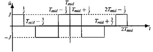
Figure 7. PARTIALLY COLLAPSED JERK PROFILE (CF. 1)
